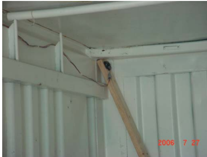
Figure 1. Experimental settings inside the container: hydrogen sensor located at the corner of the container.
