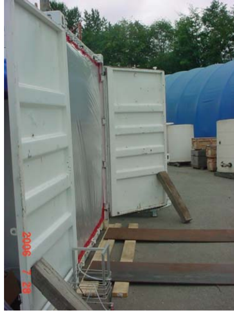
Figure 4. Plastic sheet covering perimeter of the door opening of the container.
